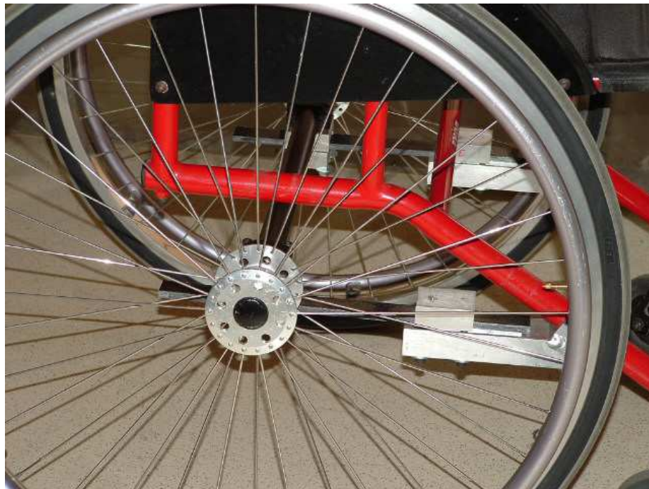
Figure 6: Composite Spring Suspension System Mounted on a Rigid Frame Wheelchair
