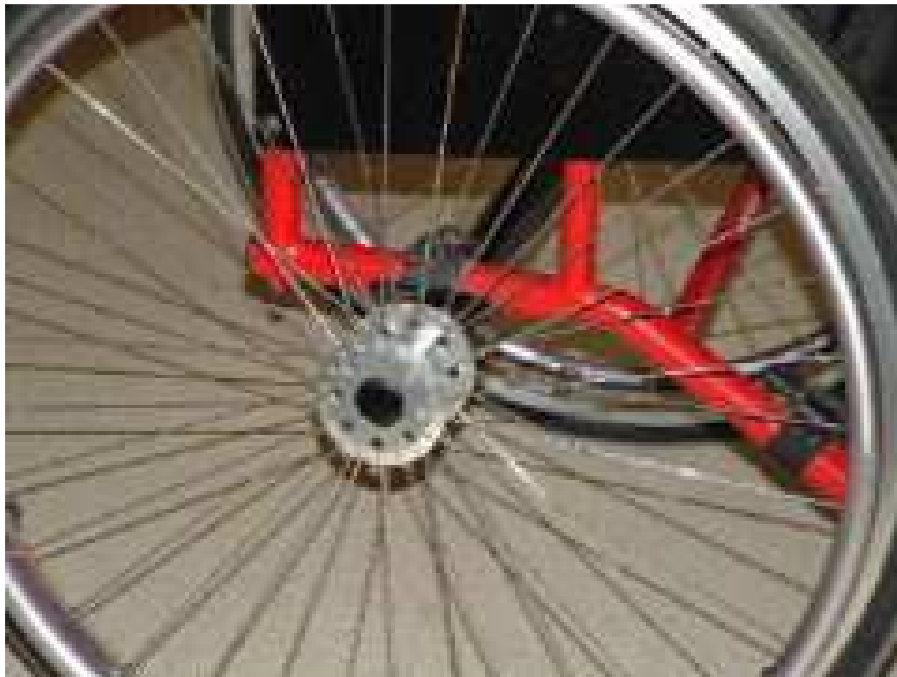
Figure 1: Non-Suspension “Rigid Mount” of the Rear Wheels on a Wheelchair
