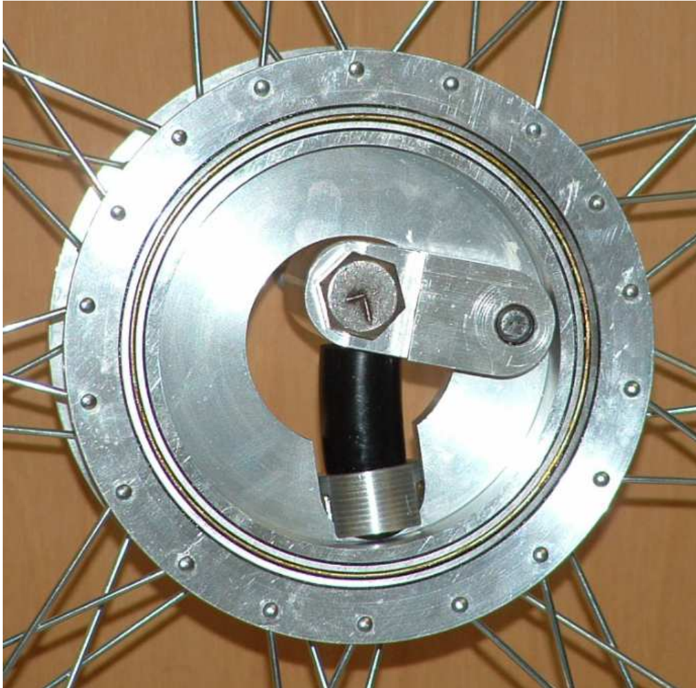
Figure 42: The Polyurethane Causes the Fork to Rotate Upward When there is No One in the Wheelchair
