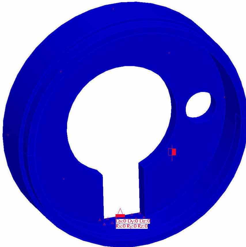
Figure 29: FEA Model of the Inner Hub, Cut in Half
